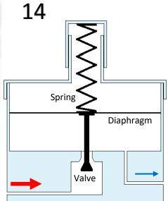
Inlet from cylinder HIGH PRESSURE Outlet to machine LOW PRESSURE The pressure regulator:
