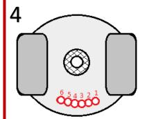
The yoke also prevents a cylinder being attached to the wrong inlet via the **Pin Index Safety System.**
